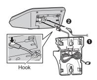
Insert the hooks on the wall mounting adaptor into the holes  $oldsymbol{\Delta}$ and **3** on the base unit.
